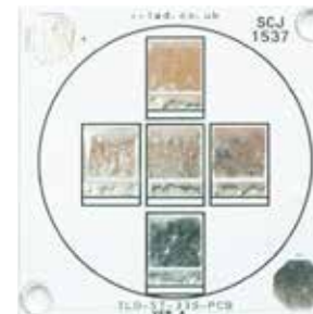
ILO-5T-33S-PCB VER A S10 X5 SERIES LES 33 SCOB Circa 7000 Lumens
