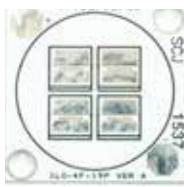
ILO-4F-19P-PCB VER A S8 X2 SERIES, X2 PARALLEL LES 19 SCOB Circa 2000 Lumens
