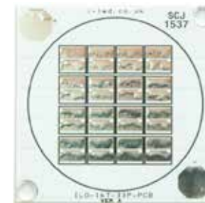
ILO-16F-33P-PCB VER A S8 X4 SERIES, 4 PARALLEL LES 33 SCOB Circa 8000 Lumens
